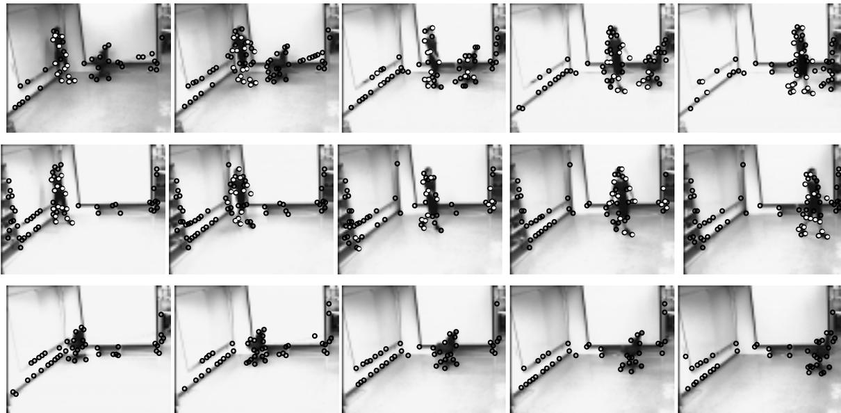
Figure 4. **Sample frames** from body and chair moving sequences (top row), body moving sequences (middle row), and chair moving sequences (bottom row). The dots (either in black or in white) are the features selected by Tomasi-Kanade algorithm on two frames. The white dots are the most human-like configuration found by our algorithm.
