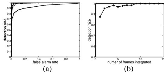
Figure 8. **Results of integrating multiple frames**. (a) Four curves are ROCs of integrating 1 to 4 frames respectively. The more frames integrated, the better the ROC curve is. (b) detection rate (when  $P_{detect} = 1 - P_{false-alarm}$ ) vs. number of frames used.
