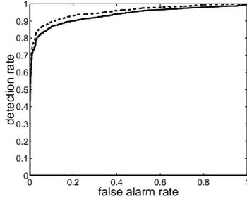
Figure 6. **ROC curves** of the detection experiment in section 4.4. Solid line: images with body and chair vs. images with chair only, the detection rate is 87.54% when  $P_{detect} = 1 - P_{false-alarm}$ ; Dashed line: images with body only vs. images with chair only, the detection rate is 89.61% when  $P_{detect} = 1 - P_{false-alarm}$ .
