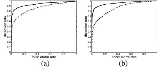
Figure 7. **ROC curves**. (a) Results of images with body and chair vs. images with chair only. (b) Results of images with body only vs. images with chair only. Solid line: using method in section 3.3; dashed line: using method in [11].
