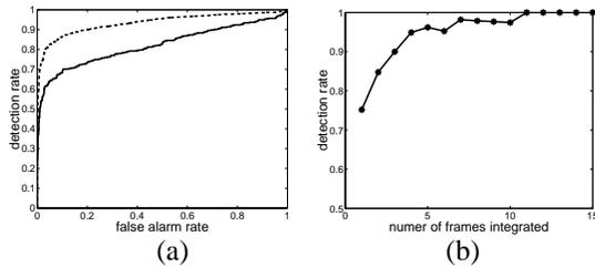
Figure 9. **Results on a different subject.** (a) ROC curves. Solid line: another subject (different from training set); Dashed line: Subject of the training set (the same as the solid line of Figure 6). (b) detection rate (when  $P_{detect} = 1 - P_{false-alarm}$ ) vs. number of frames used for the new subject.
