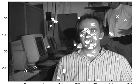
Figure 2: Candidate feature locations produced by the detectors: left eye-o, right eye-o, nose/lip-*, left nostril+, right nostril-x.
