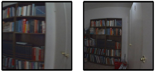
Fig. 3. The current view from the camera (left), which is successfully matched with the landmark image (right).
