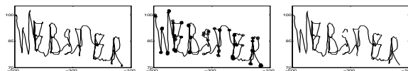
Figure 2. (a) trajectory obtained for the sequence “Webster”, (b) segmentation points (marked with ‘o’), (c) shows the resulting segments.
