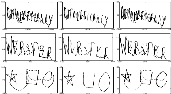
Figure 6. Results of the classification algorithm on the several sequences of the database using 15-NN. The trajectories obtained with the pen tip tracker are shown in the first column. The segments classified as pen down are shown in the second column. The plots in the third column display segments with a thickness is proportional to the confidence in the classification, where the confidence is the percentage of votes for pen down out of the total number of votes. ‘-’ pen down segments and ‘- -’ pen up segments.
