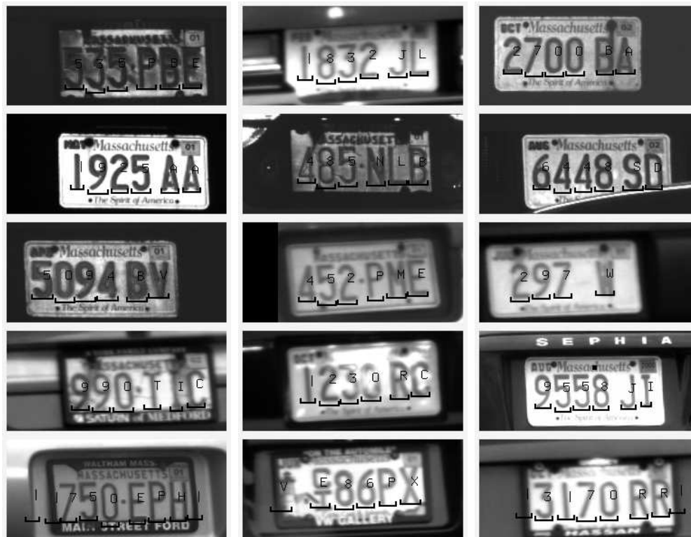
Fig. 11. Examples of detections on a variety of plates. Last rows illustrates false positives
