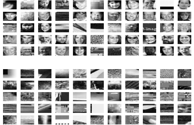
Figure 4: A subset of the training data, face examples (top) are contaminated with wrongly labeled non-faces, non-face examples (bottom) are random patches cut from images not containing the target. Face data may also contain within-class outliers - correctly labeled but hard to learn examples.
